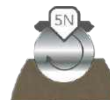
Coupe-Test (Blade Cut Resistance)
